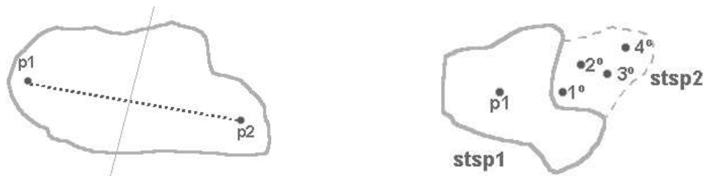
Fig. 2. On the left, we select p_1 and p_2 , and then divide the set. On the right, the merge step takes the objects according to their distances towards p_1 .
